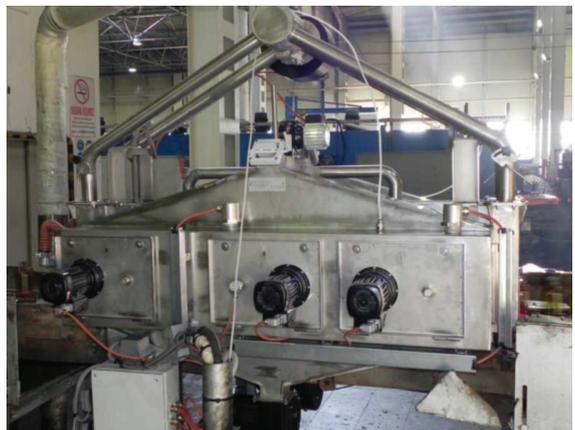
GlassChem HECSt 1800 hot end coating system has been developed specifically for high speed production lines.
