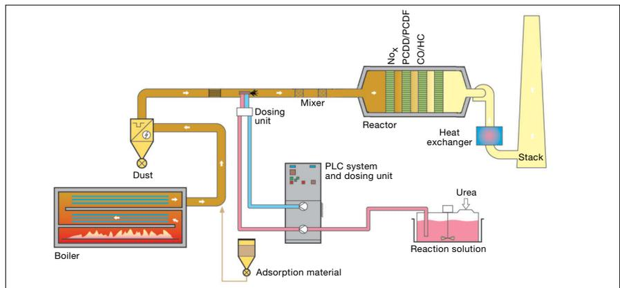
Catalytic waste gas purification for thermal waste utilization
