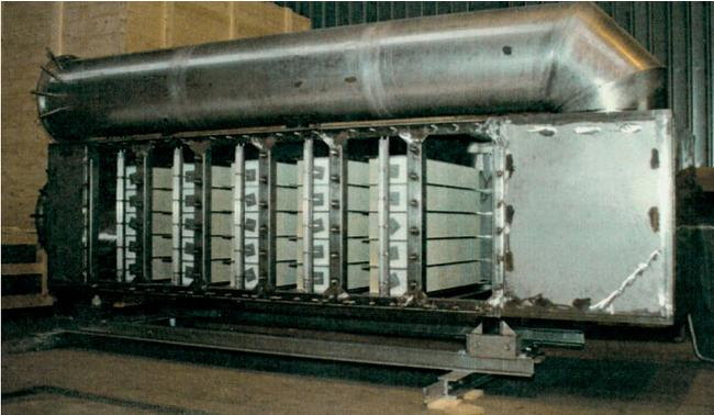
Catalytic reactor with 6 rows of catalyzers for pickling plant
