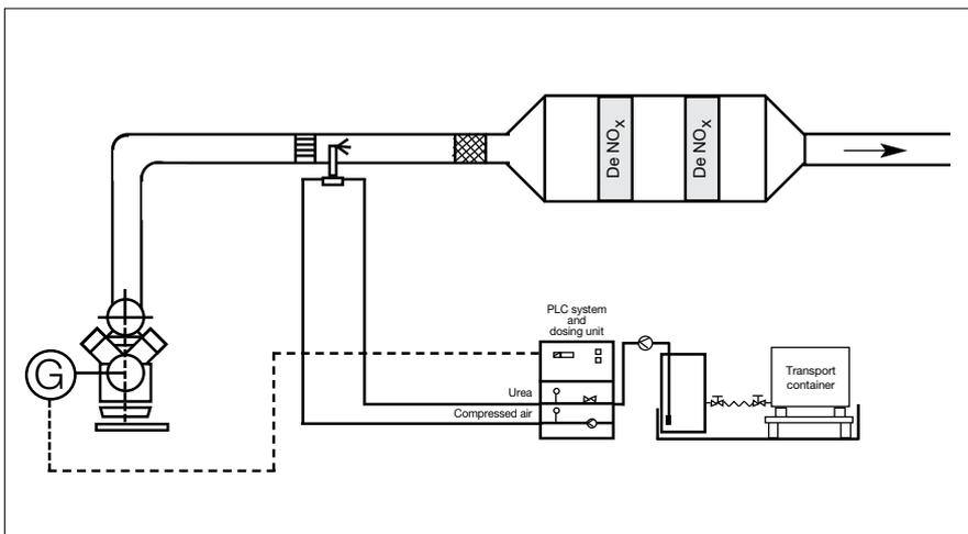
SCR catalytic converter for engines
