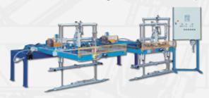
Automatic Push-Bar, designed to transfer the printed items from the machine conveyor to the lehr. The unit can be designed in a single or double independently controlled units.
