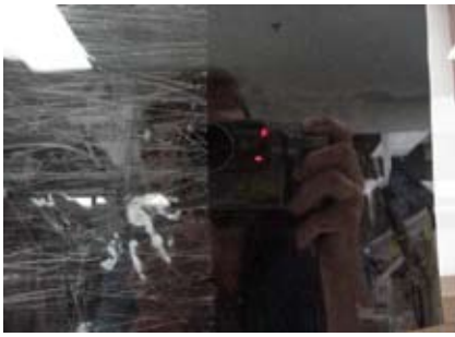
Figure 6 Surface damage on half-coated glass, caused by repeated contact with glass and metal objects.
